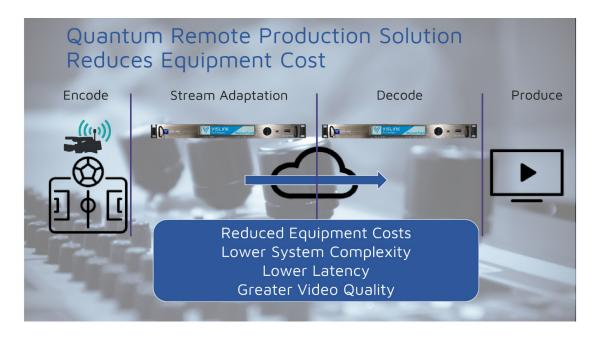
With much focus on high quality 4k and HDR formats, the removal of a stage of encode-decode compression concatenation can increase video quality and help to ensure that the wireless camera provides video quality excellence to complement line cameras that might make up the rest of the camera views.
