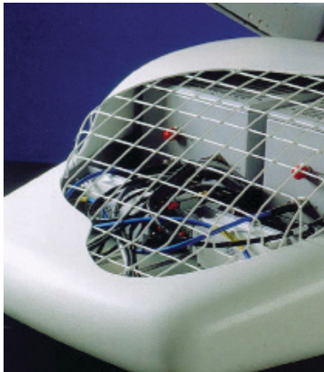
Two HPAs located within the antenna assembly
