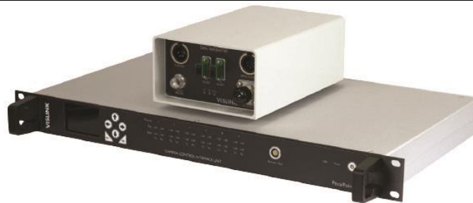
Figure 1-1 FocalPoint Wireless Camera Control System
