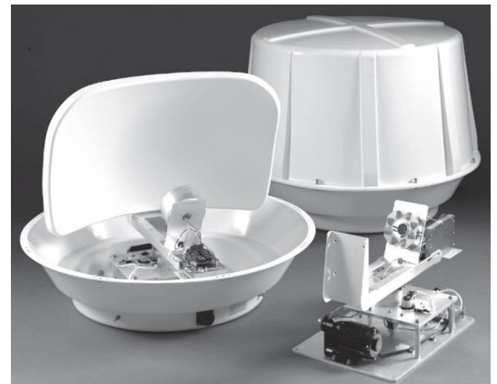
UltraScan Antenna with Radome Removed
