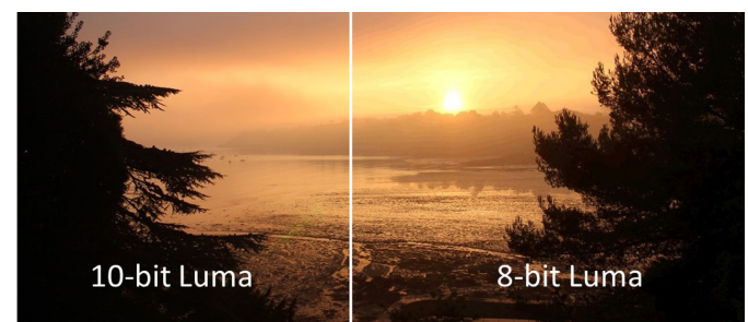
Figure 3 How 8-bit luma video suffers posterization artefacts compared to 10-bit luma video
