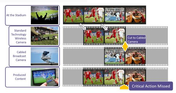
Newer, more sophisticated HEVC UHD capable wireless camera systems have recently been developed that significantly reduce processing latencies. By improving the video decode implementation through optimized buffer management and implementing greater parallel processing by pipelining the data flows, end-to-end latencies as low as a single video frame can be achieved.
