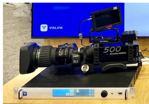
Figure 2: High Frame Rate Camera in Combination with Vislink Cliq Transmitter and Quantum Receiver
