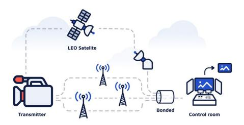
Through intelligent channel bonding algorithms, not only is transmission data spread across all available connections, but additional error correction and retransmission mechanisms work tirelessly to ensure connection robustness.
