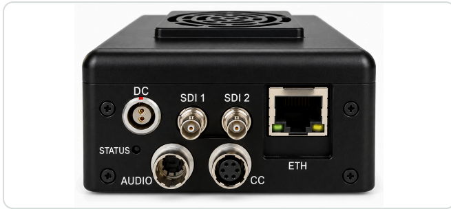
Camera side: DC, SDI 1/2, Audio, CC, ETH and status LED
