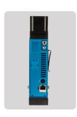
LiveLink sets a new standard in bonded cellular technology, delivering market-leading video quality with ultra-reliable, low-latency transmission. Designed for versatile mobile camera applications, LiveLink supports 4x HD or 1x UHD 4:2:2, 10-bit HEVC HDR video encoding, making it ideal for everything from multicamera sports broadcasts to critical live events
