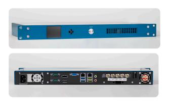
The Vislink Q-Link is an integral component of the Airborne Video Downlink System (AVDS). The Q-Link controls, aggregates, and distributes video captured from airborne platforms to multiple observers over secure IP networks. The Q-Link extends critical situational video to an unlimited number of observers.
